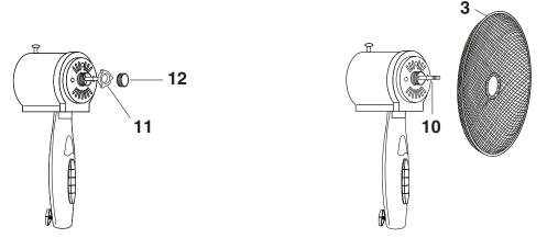
2 Fit the propeller (2) onto the motor shaft (10) and secure it with the threaded cap (12). The screw cap has the opposite left thread.
