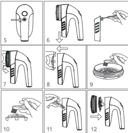
5. Clean the dirt in the planchet with the supplied cleaning brush (fig. 9).
