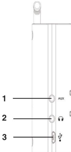
1 3.5 mm **AUX** mini connector (external audio device connection)
