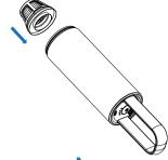
3 Disassemble the filter assembly by turning the filter basket counterclockwise and pulling out the filter basket. Shake the filter housing itself and shake off the dirt. Parts and filter can be rinsed with water. Both parts and filter must dry completely before reinserting. If necessary, replace the filter housing with a new one.
