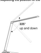
You can adjust the position of the lamp head and arm in a range of 225°. You can adjust the inclination of the lamp arm in the range of 90°.
