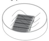
3 Replace the filter and press and hold SLEEP/RESET reset the filter counter.
